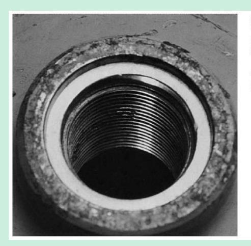
PHOTO 5. Damaged threads.
