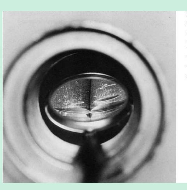
PHOTO 15. Fold near the thread region. Mirror view shows clearly that the fold does not enter into the full-thread area. This type of fold is acceptible if the depth of the fold is estimated to be less than 0.060 inch (1.53 mm).
