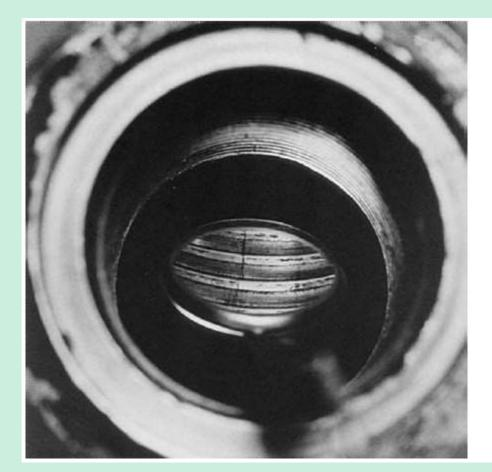
**PHOTO 7.** A crack in the threads found by the use of a dental mirror.
