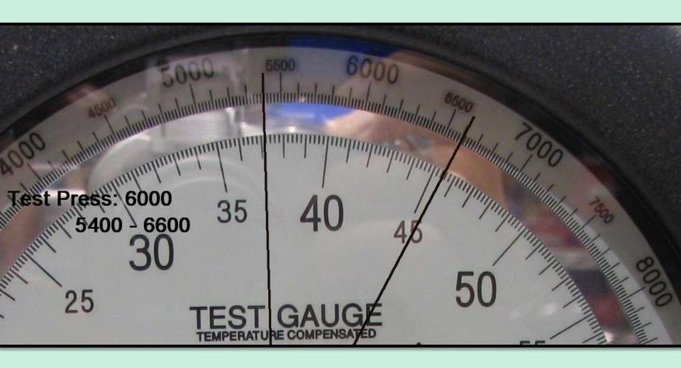
of each cylinder tested, except that for an analog device, interpolation to ½ of the marked gauge divisions is acceptable. The expansion-indicating device of the testing apparatus must also permit incremental reading of the cylinder expansion to 1% of the total expansion of each cylinder tested or 0.1 cc, whichever is larger. Midpoint visual interpolation is permitted.
