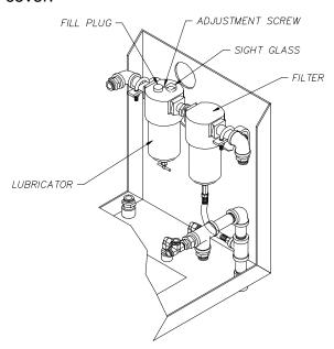
Figure 6-1 Air Motor Lubricator
