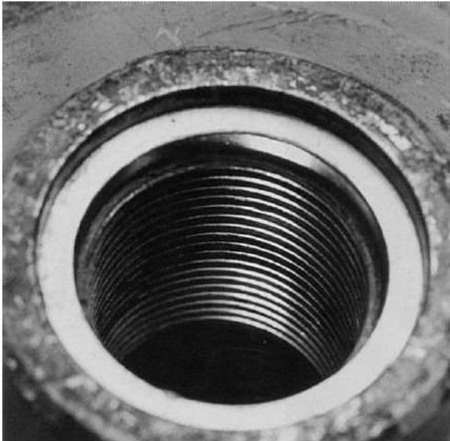
**PHOTO 19.** Dirty and worn threads. The threads at the bottom are worn and not as 'sharp' as the threads near the top. The threads need to be cleaned before counting the good threads (starting from the top).
