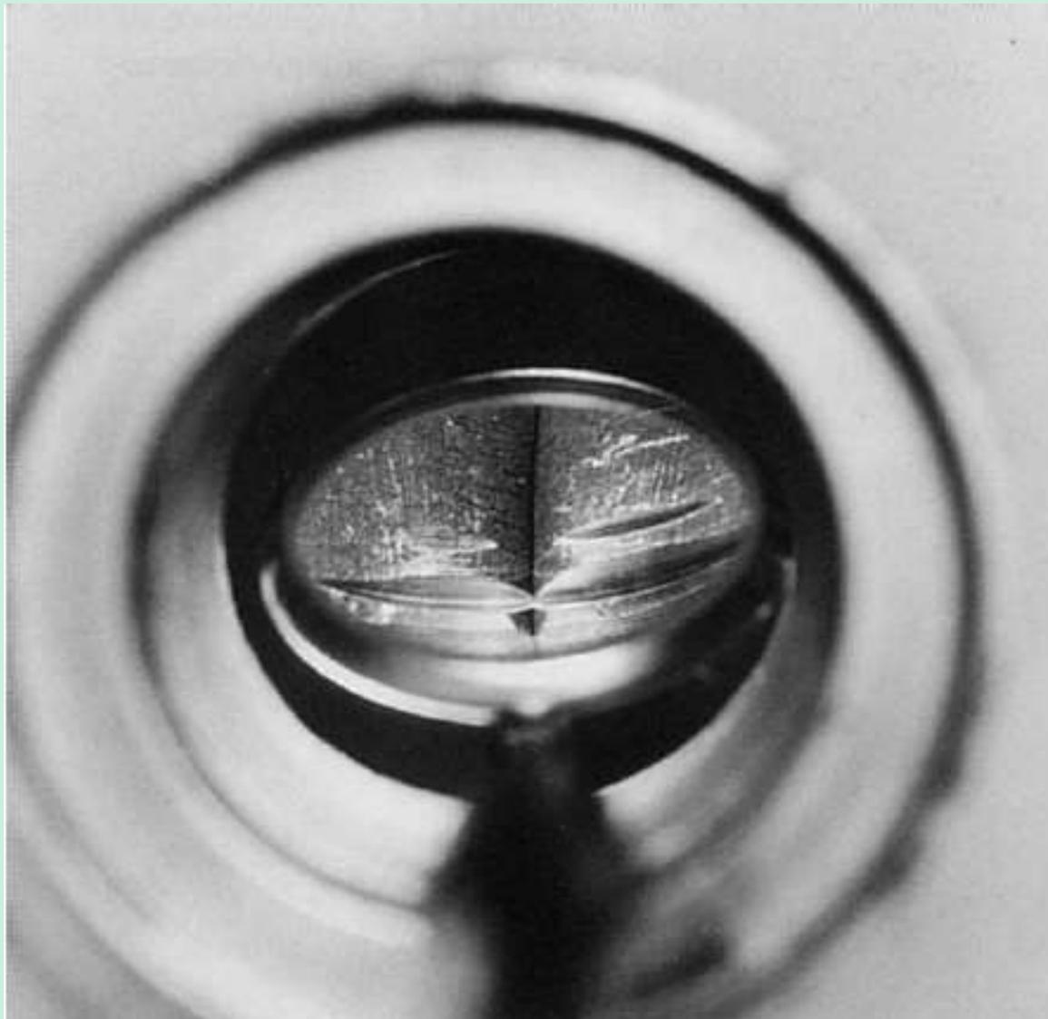
**PHOTO 15.** Fold near the thread region. Mirror view shows clearly that the fold does not enter into the full-thread area. This type of fold is acceptable if the depth of the fold is estimated to be less than 0.060 inch (1.53 mm).
