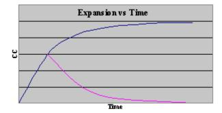
The graph shows the expansion gradually reaching a steady value. It can be plotted either as the expansion value itself (in which it tends to reach a stable value) or as the change from the last reading - this will tend towards zero. Values could be increasing or decreasing. A straight line or steady expansion change over time represents a leak - not a temperature effect!
